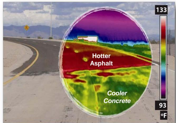
**Figure 3. Thermograph of a highway in Mesa, Arizona, illustrating the temperature difference between concrete and asphalt pavements.**
