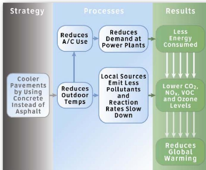
Figure 1. Ways in which concrete pavements can indirectly save energy, improve air quality, and combat global warming. [After: Akbari]
