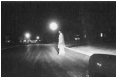
Asphalt roadway showing limited surface reflectance
