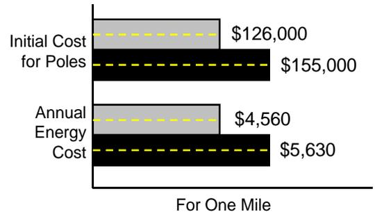
Assumes: Initial cost = \$5,000/pole; Maintenance cost = \$100/pole/year; Energy cost = \$0.0814/kwh; Operating time = 4,000 hours/pole/year
